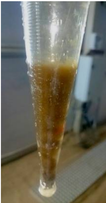
Imhoff cone showing biofloc settled
